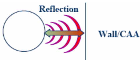
Fig. 7. Proximity sensors operating on the principle of reflections from wall and other CAAs
