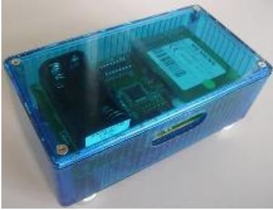
Fig. 7. Siemens "Blue Box" with BTnode, A80 target node and batteries. The Adapter Board acts as a connecting cable.
